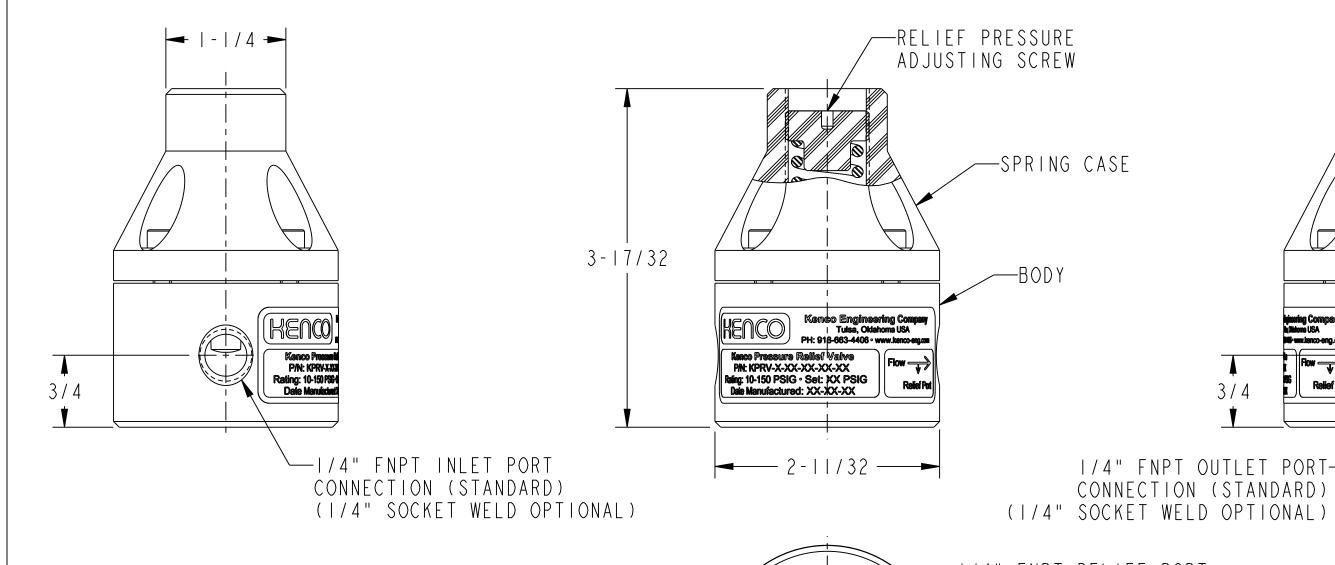
RELIEF PRESSURE ADJUSTMENT RANGE: 0 TO 150 PSI RELIEF PRESSURE FACTORY SETTING: 50 PSI
