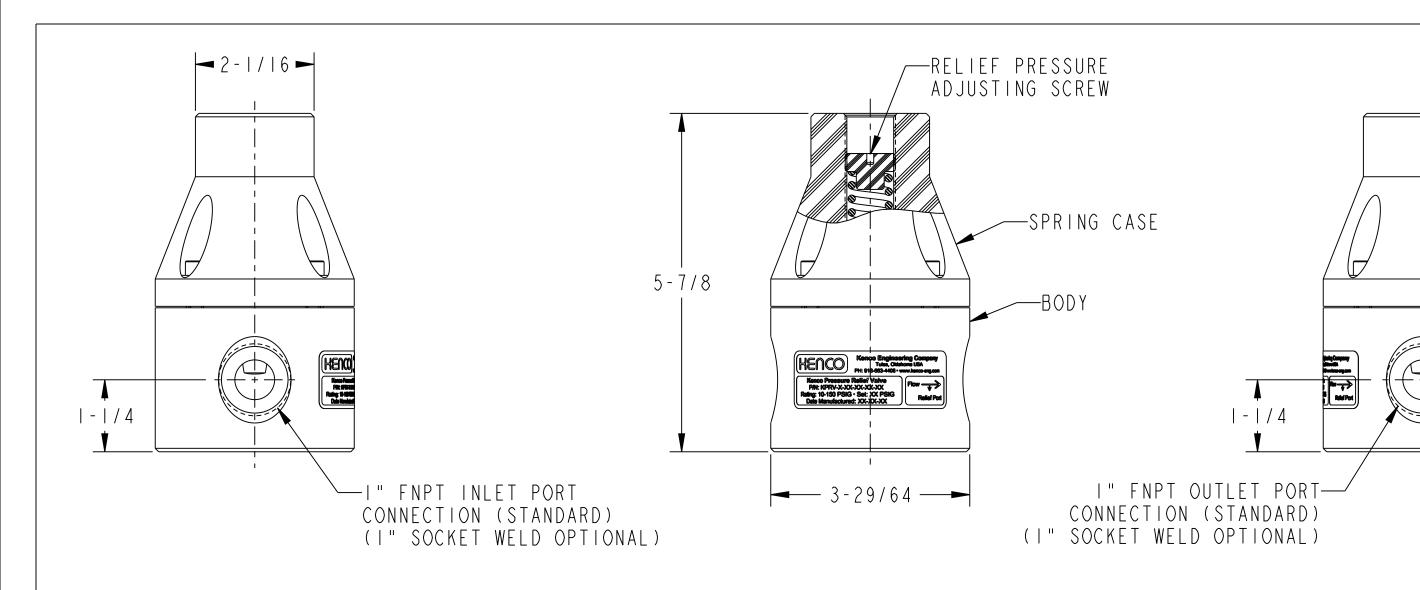
RELIEF PRESSURE ADJUSTMENT RANGE: 0 TO 150 PSI RELIEF PRESSURE FACTORY SETTING: 50 PSI
