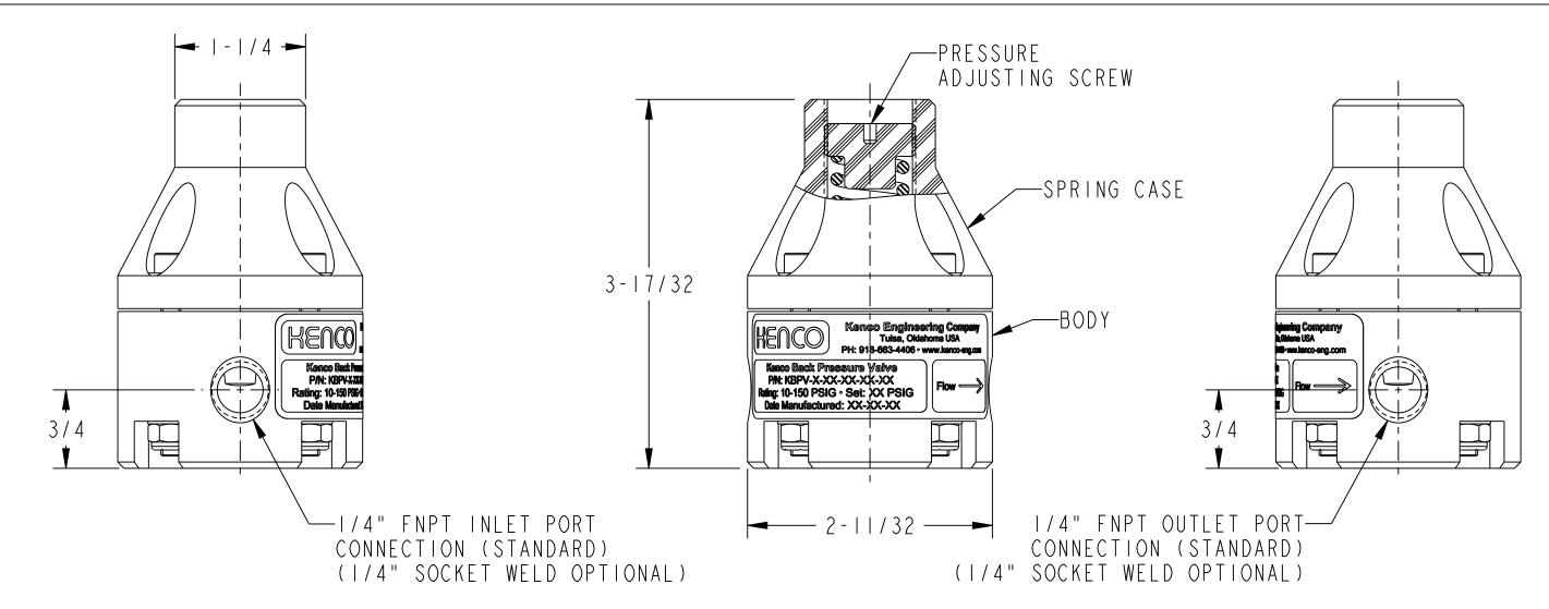
RELIEF PRESSURE ADJUSTMENT RANGE: 0 TO 150 PSI RELIEF PRESSURE FACTORY SETTING: 50 PSI
