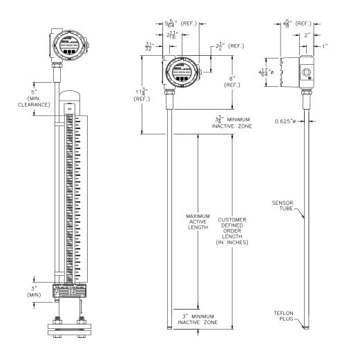
Note: In a typical application, KENCO adds 2 inches to the order length so that the customer has additional mounting flexibility. Units are factory calibrated with the additional 2 inches at the top of the gauge, bringing the total inactive zone at the top to 7".
