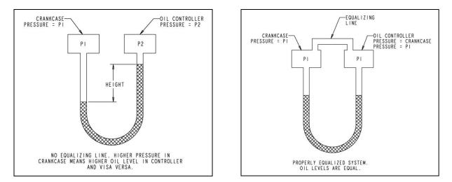
• A pressure difference of 0.032 psi will result in an oil level difference of 1" between the oil controller and the crankcase when using 40W oil with a specific gravity of 0.89. 0.064 psi would be 2"; 0.128 psi would be 4" and so on. 1 psi pressure difference results in an oil level difference of 31"! This large effect on the oil level resulting from such a small difference in pressures is why proper equalization is so important.
