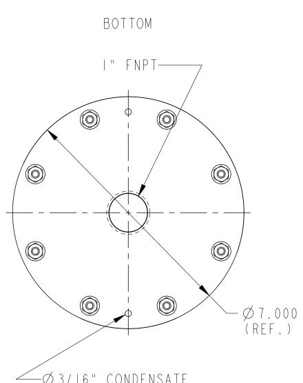
$-\phi$  3/16" CONDENSATE DRAIN HOLE (2 PLACES)
