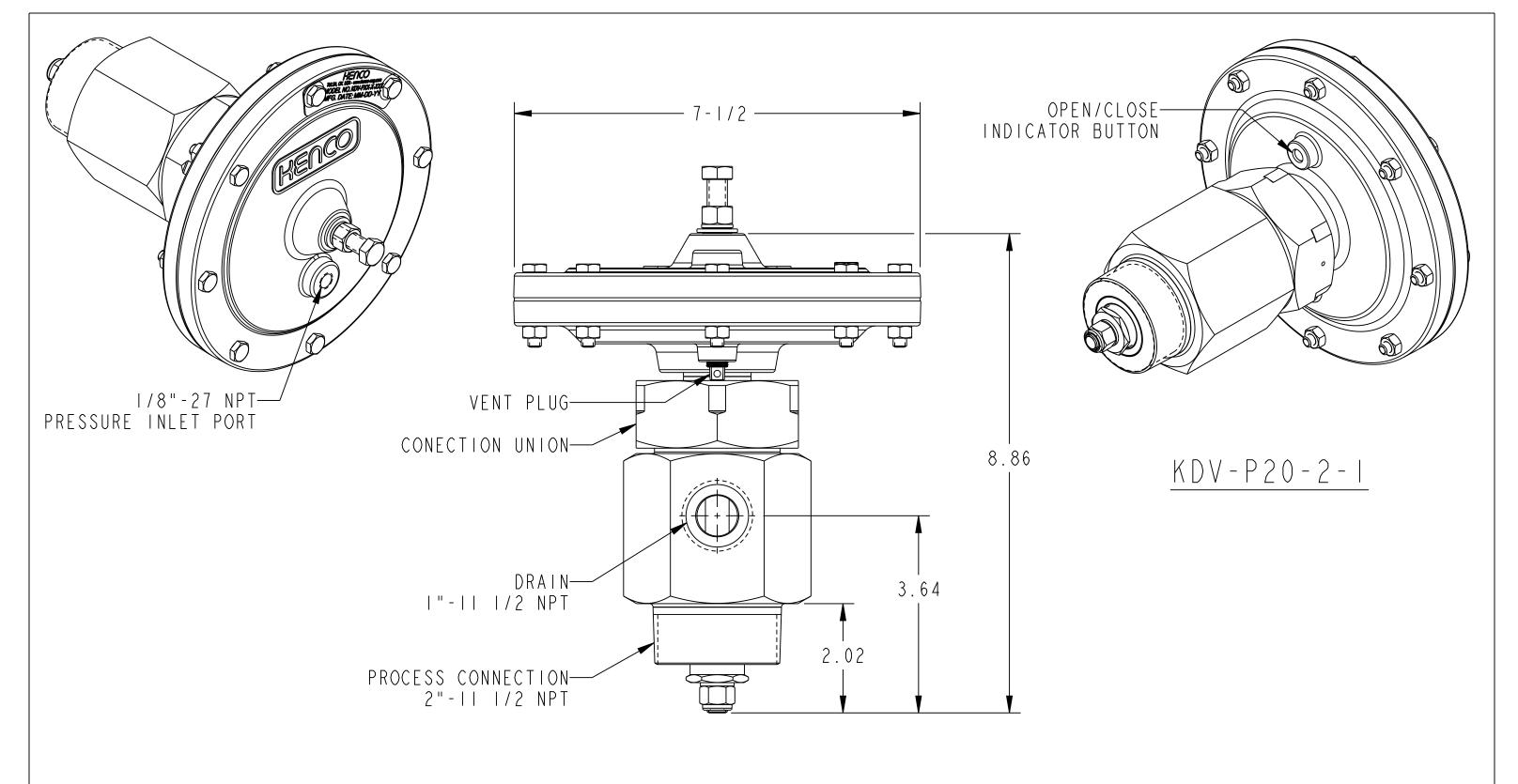
PRESSURE RATING: 2000 PSI MAXIMUM VALVE RELEASE PRESSURE: 70 PSI
