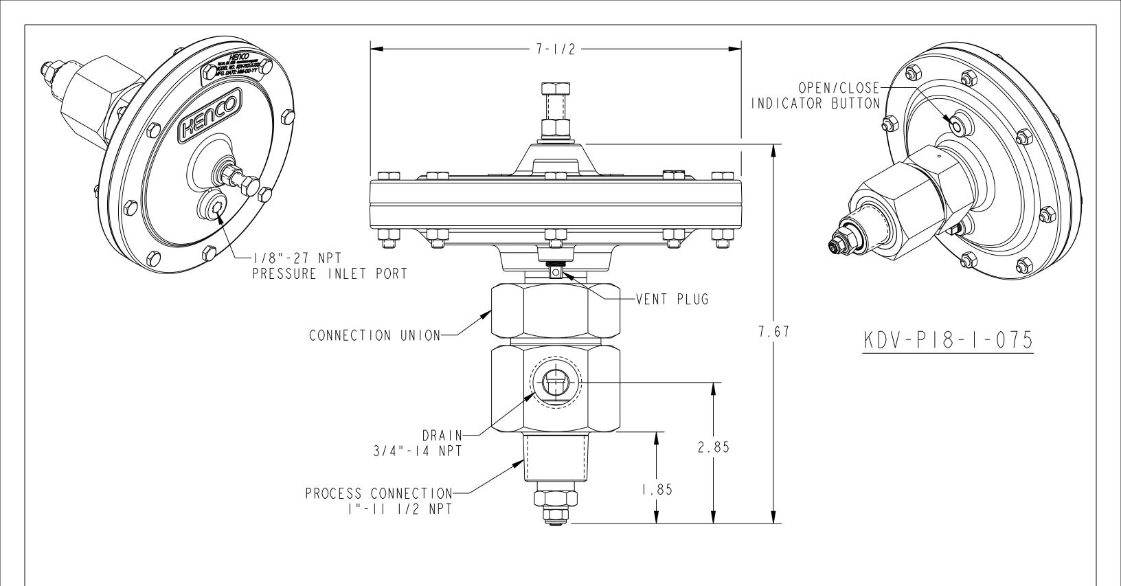
PRESSURE RATING: 1800 PSI MAXIMUM VALVE RELEASE PRESSURE: 45 PSI
