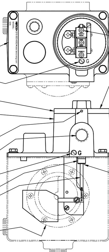
6-32UNC Binding Head Switch Terminal Screws with Cup Washer
