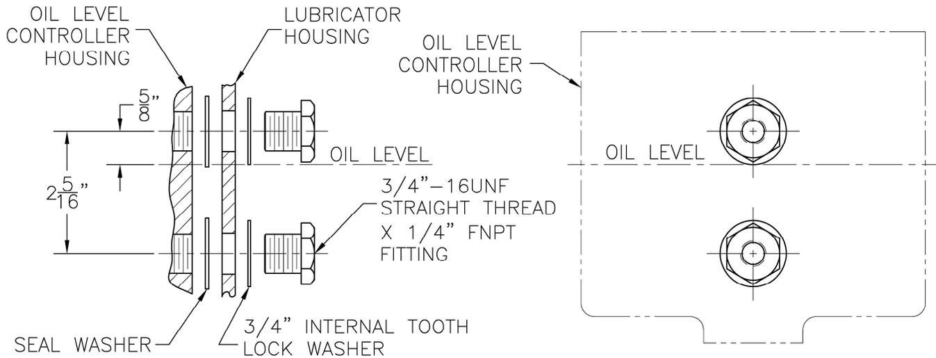
(Drill 25/32"Ø holes in lubricator housing to mount)
