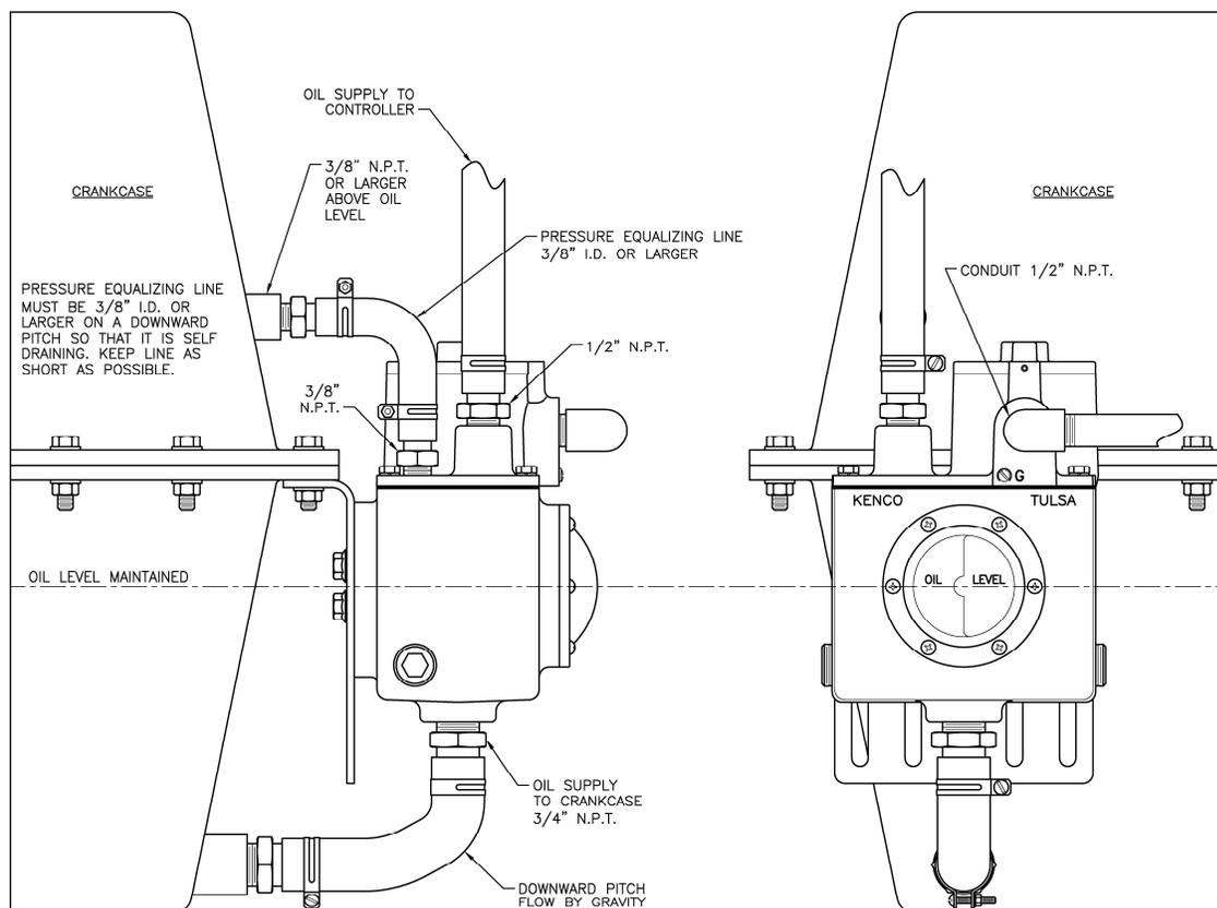
**FIGURE 2: MECHANICAL LUBRICATOR -11 AND -11-FS OPTION**
