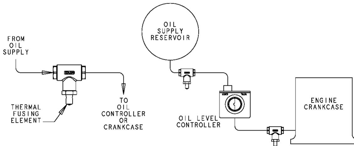
**Note:** Flow on the KFS valve is bidirectional. Either port can serve as the inlet or outlet.
