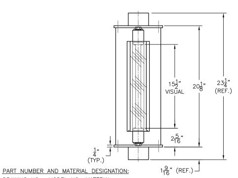
DRAWING NO. C-15854-CS MODEL NO. 15854-CS (CARBON STEEL TANK WITH 316/316L STAINLESS STEEL WETTED PARTS ON SIGHT GAUGE)
