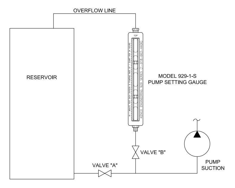
If top of gauge is below the maximum operating level of liquid in tank or if any negative or positive pressures exist, the 1/4" FNPT upper equalizing line connection in gauge should be connected to upper part of reservoir with a vent tube having a 5/16" minimum inside diameter.
