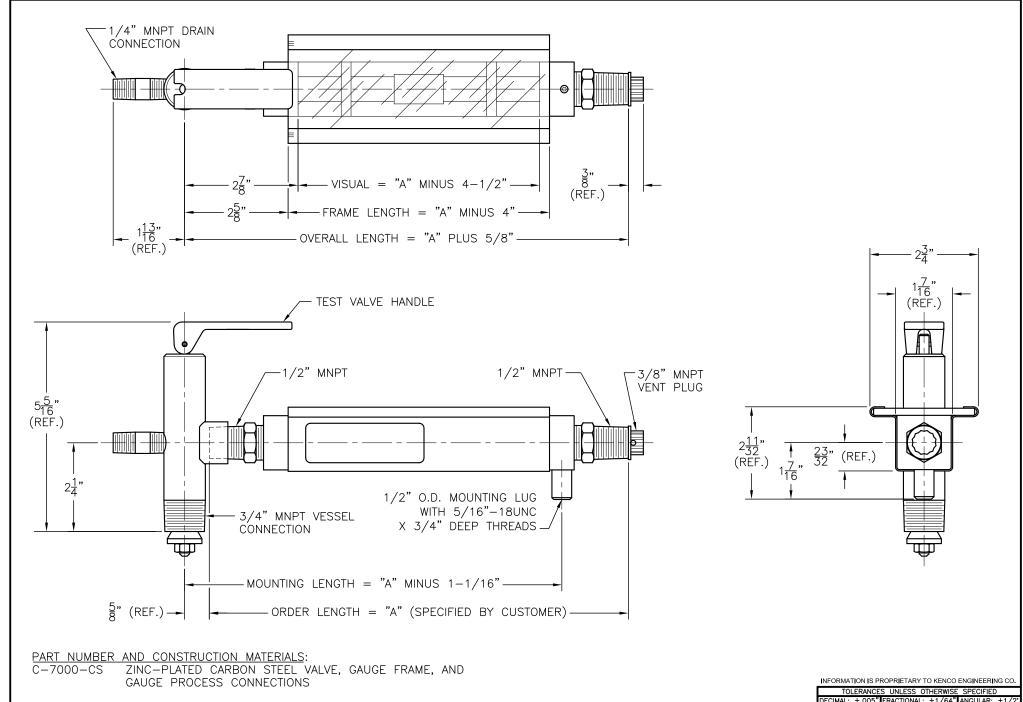
C-7000-SS 304 STAINLESS STEEL VALVE AND GAUGE FRAME WITH 316 STAINLESS STEEL GAUGE PROCESS CONNECTIONS
