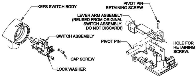
(Note: Some early model of the KEFS used a Clevis Pin and Hitch Pin to retain the Lever Arm assembly. If this is the case with your KEFS, you will not be able to use the Pivot Pin with the Pivot Pin Retaining Screw since the Lever Arm in these early units did not have the hole for the Retaining Screw. If you have one of these early units simply discard the Pivot Pin and Pivot Pin Retaining Screw included in the kit and reuse the Clevis Pin and Hitch Pin.)
